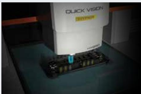
Example of measuring an engine control unit
