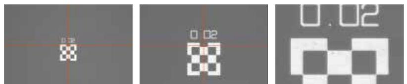
Turret 1X Field of view: 0.62×0.47 mm      Turret 2X Field of view: 0.31×0.23 mm      Turret 6X Field of view: 0.10×0.07 mm
